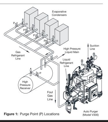
A higher temperature measured at this point, compared to the saturation pressure, indicates the presence of non-condensable gases in the system.
