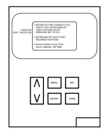
Figure 9: Control Panel - Displaying Initial Startup Screen
