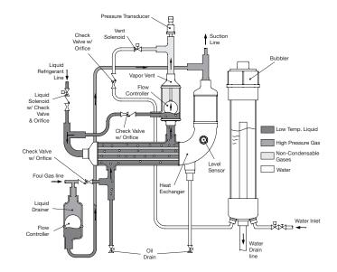
\*Figure 3: Purger Separation of Non-Condensable Gases & Refrigerant Cycle
