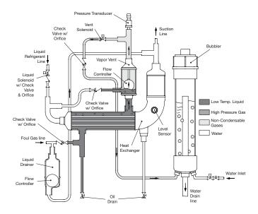
\* Figure 4: Purger Release of Non-Condensable Gases
