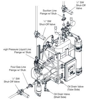
Figure 6: Purger Flange Line Connections
