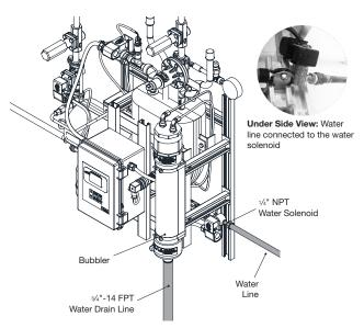
Figure 7: Water Line Connections
